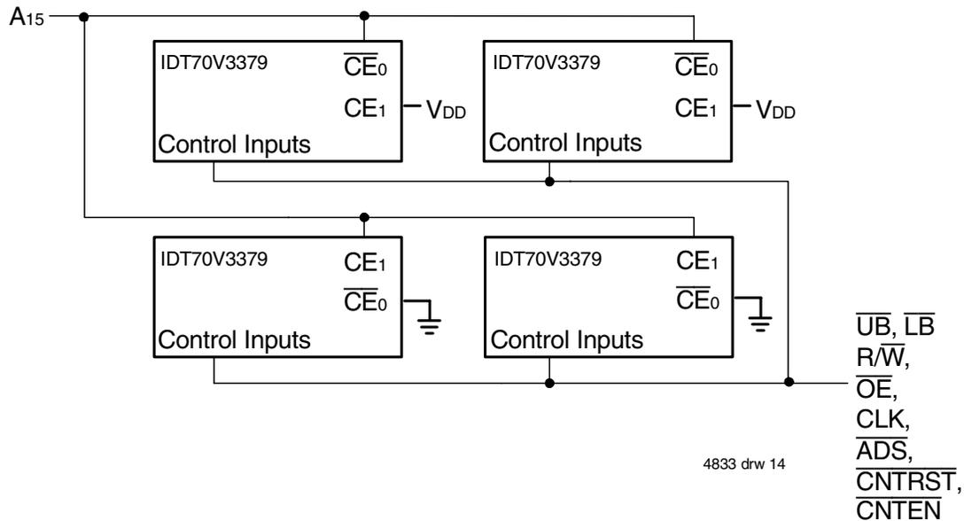
Figure 4. Depth and Width Expansion with IDT70V3379
