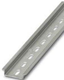
DIN rail perforated, Standard profile, width: 35 mm, height: 7.5 mm, acc. to EN 60715, material: Steel, galvanized, length: 2000 mm, Hole size: 5.2 mm x 18 mm, color: silver
