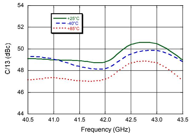
**Typical Performance Curves:  $V_D = 4\text{ V}$ ,  $I_{D1} = 217\text{ mA}$ ,  $I_{D2} = 300\text{ mA}$ ,  $I_{D3} = 600\text{ mA}$ ,  $T_A = 25^\circ\text{C}$**
