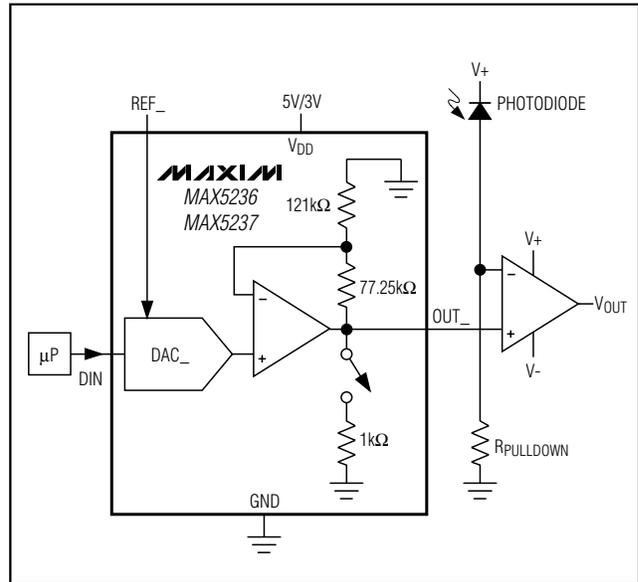
Figure 10. Digital Calibration
