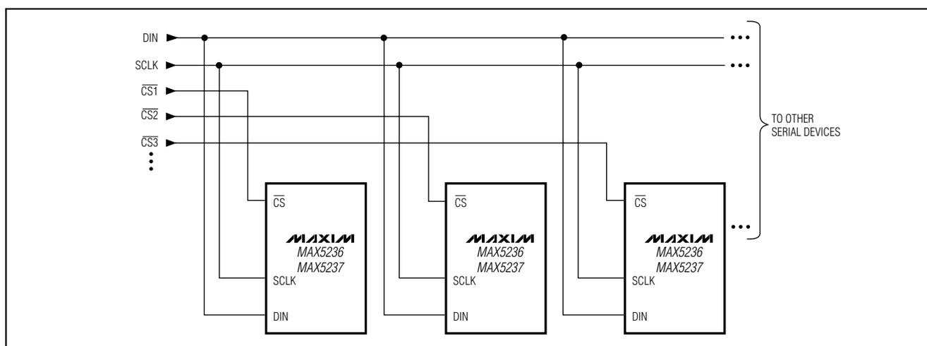
Figure 12. Multiple MAX5236/MAX5237 Sharing a Common DIN Line
