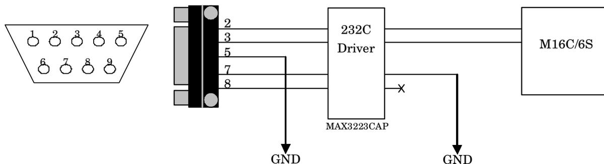
**Figure 6: Connection diagram of J1**
