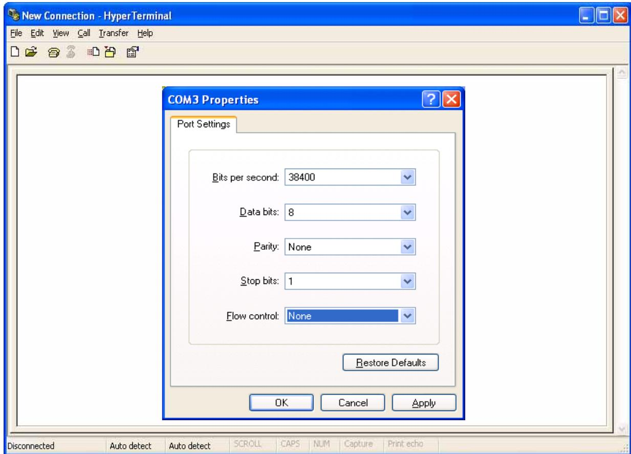
The COM setting window will be cleared, and only the terminal window will remain on the desktop. After that, push the reset switch of EV5 once. The program for simple communication tests will be started, and the following messages shown on the next page will appear on the terminal window.
