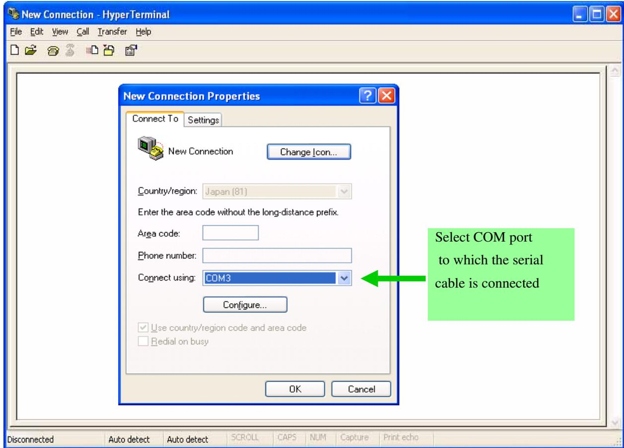
After checking that the COM port to which the serial cable is connected is selected as “Connect using”, click “OK”. Then the sub window as shown below will appear. Set each COM port condition as follows and click “OK”.
