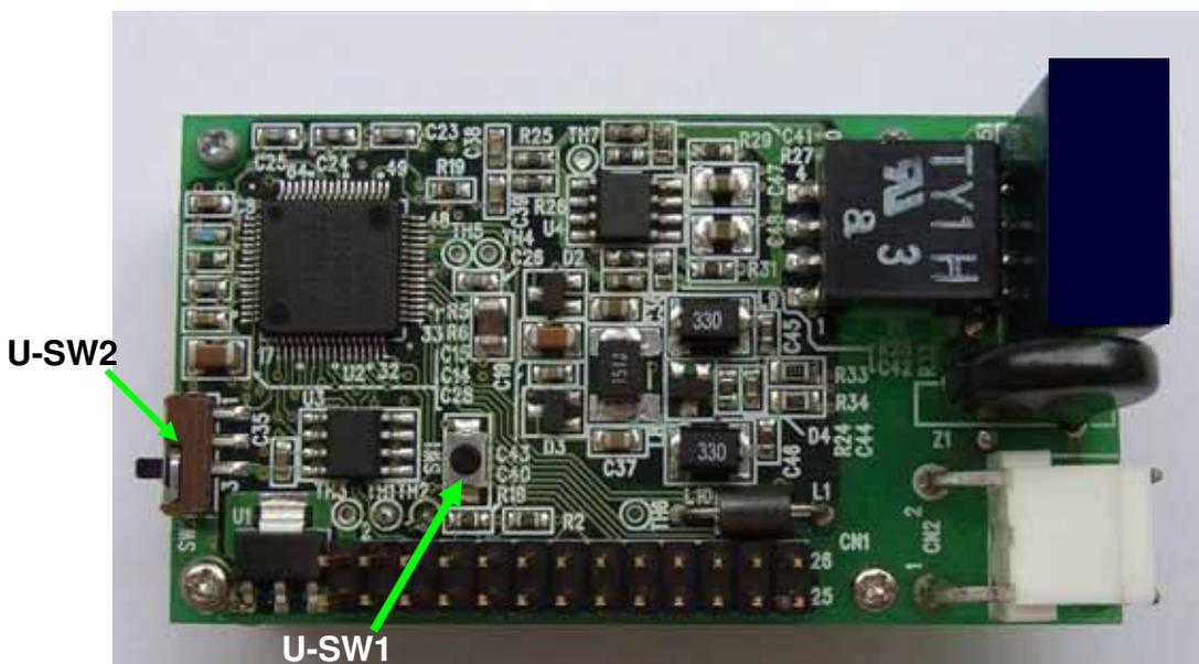
**Figure 7: Location of switches on the upper board**
