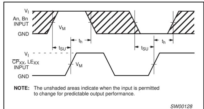
Waveform 4. Data set-up and hold times for the An and Bn inputs to the LE<sub>AB</sub>, LE<sub>BA</sub>, CP<sub>AB</sub> and CP<sub>BA</sub> inputs
