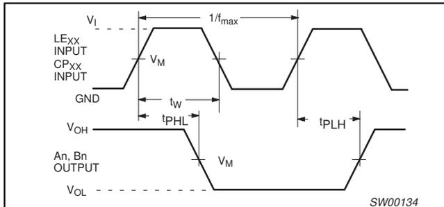
Waveform 2. Latch enable input (LE<sub>AB</sub>, LE<sub>BA</sub>) and clock pulse input (CP<sub>AB</sub>, CP<sub>BA</sub>) to output propagation delays and their pulse width
